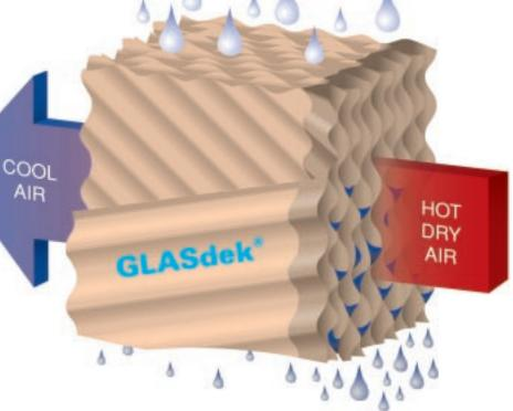
The steeper angle directs more water to the air entering side of the pad, where it is needed most.
